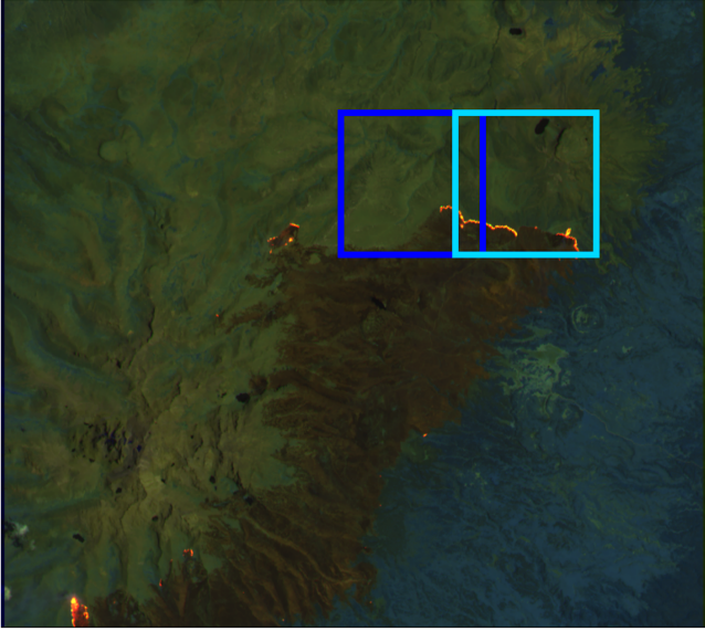
Fig. 6. Decomposition of a raw granule into 256 \times 256 patches with 25% of patch overlap.
