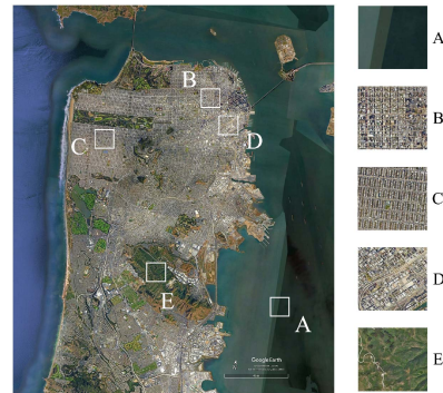
Fig. 3. Optical image of the experimental area in San Francisco, USA from Google Earth, with white squares marking five typical targets: the ocean (area A), the built-up areas with small, medium, and large polarization orientation angles (areas B, C, and D), and the vegetated region (area E).
