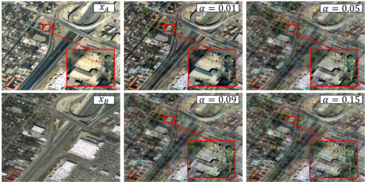
Fig. 6. Impact of varying the size of \alpha on the Fourier-based frequency transformation operation is noteworthy: As \alpha increases, the cross-temporal gap between bitemporal RSI decreases, yet it also tends to introduce artifacts, as illustrated in the zoomed insets.
