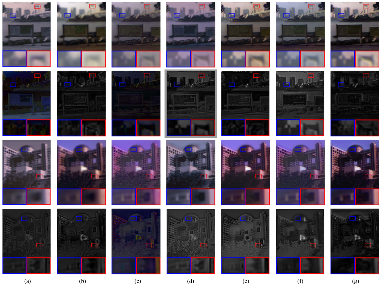
Fig. 10. Qualitative results on 24th band on Saliency dataset. First and third rows: two reconstructed images with two comparison areas were upscaled four times for clarity. Second and fourth rows: corresponding error. (a) PGCU. (b) DRPNN. (c) GDD. (d) Gppnn. (e) HyperPNN. (f) DHP-DARN. (g) HS-McHF.
