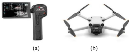
Fig. 15. Equipment used in real image acquisition. (a) Thermal imaging camera. (b) UAV.
