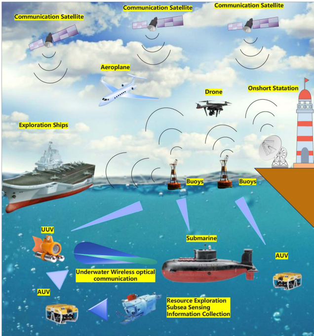
Fig. 1. Typical scenario of underwater wireless optical communication.
