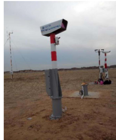
Fig. 3. Lidar for visibility measurement.
