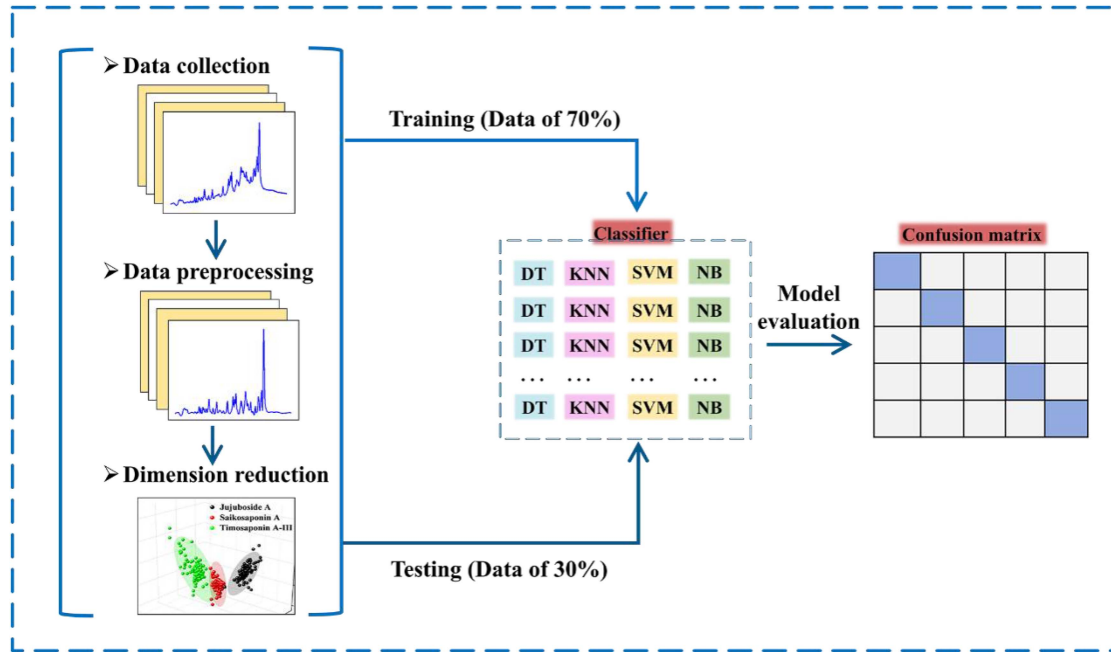
Fig. 2. Flowchart of machine learning classification algorithm.
