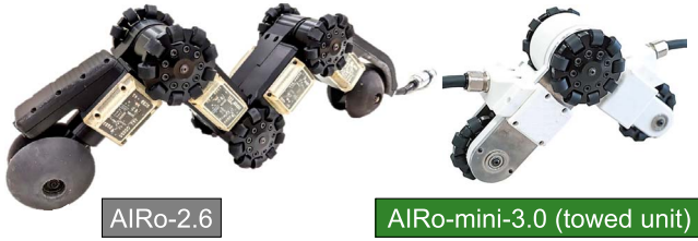
Fig. 1. Overview of the developed towed sensing system. AIRO-2.6 is a self-propelled in-pipe inspection robot and AIRO-mini-3.0 is a towed sensing unit.
