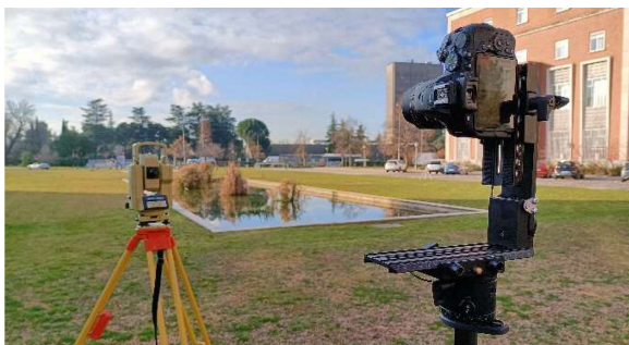
FIGURE 3. Arrangement of the reflex camera and the topographic total station used in one of the panoramic images taken (training field at ETSIAAB).
