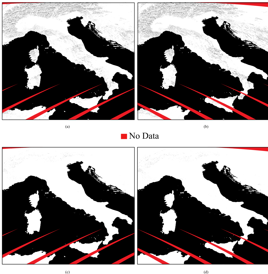
Fig. 15. Masks of geometric distortions in a 49° MIO, right-looking acquisition mode. Black areas are affected by the phenomena of geometric distortion and thus do not appear to be in the SAR visibility. (Top) Foreshortening/Layover mask for (a) ascending and (b) descending case. (Bottom) Shadow mask for (c) ascending and (d) descending case. Red areas are related to gaps in coverage (no data).
