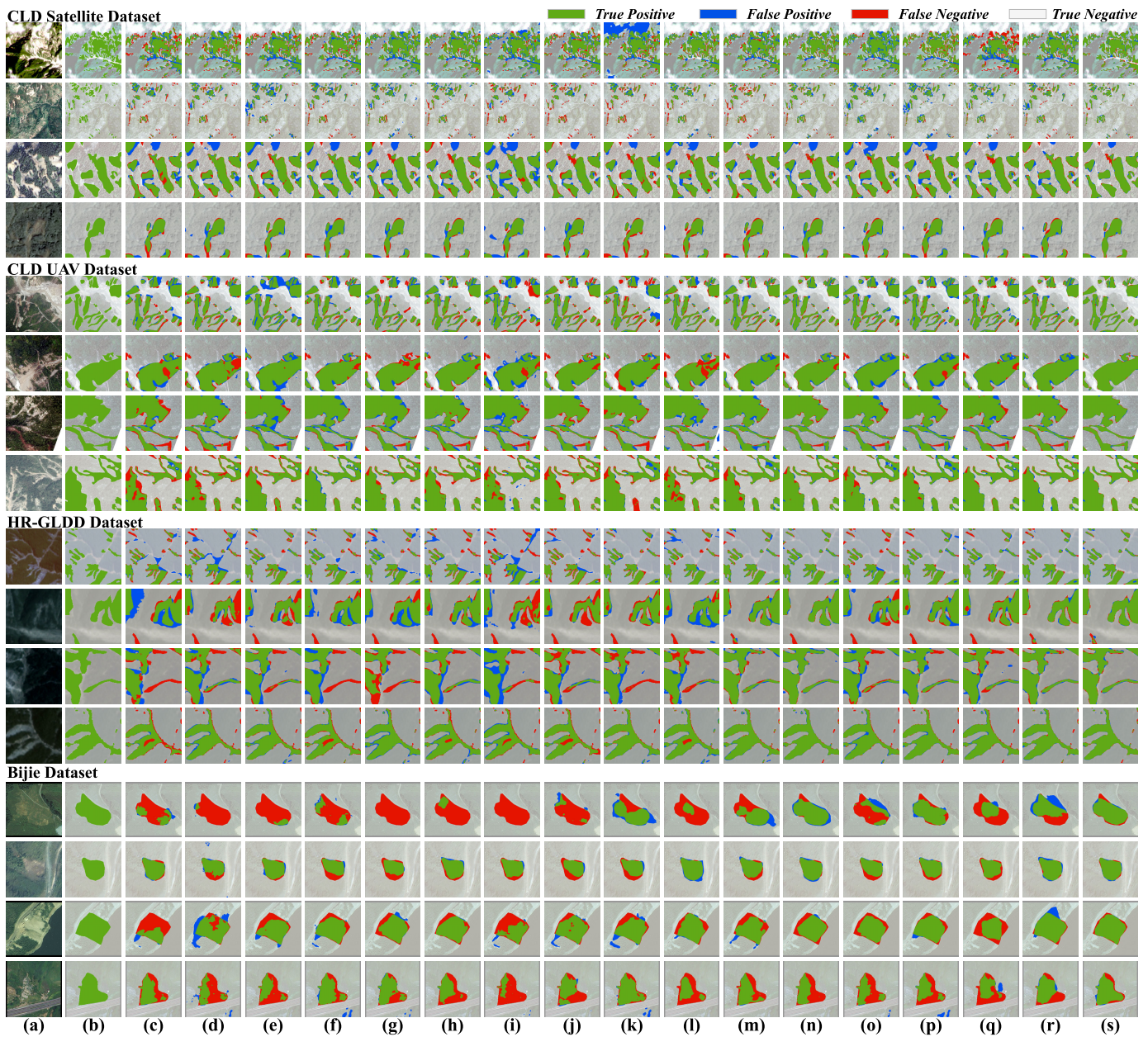
Fig. 6. Landslide detection results comparing with 16 state-of-the-art approaches across different datasets (CLD Satellite, CLD UAV, HR-GLDD, and Bijie), including traditional CNN-based methods, lightweight model, attention-enhanced methods, modern backbone network, Transformer-based models, and mamba-based model. (a) Optical RSIs; (b) GT; (c) FCN; (d) U-Net; (e) ResUNet; (f) PSPNet; (g) DeepLabv3+; (h) HRNet; (i) ICNet; (j) CCNet; (k) GCNet; (l) PIDNet; (m) DANet; (n) ConvNeXt; (o) SegFormer; (p) Swin Transformer; (q) ST-UNet; (r) VMamba; and (s) SCGC-Net (ours).
