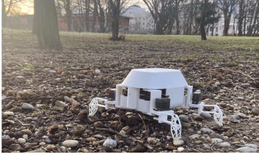
Fig. 1. Turtle-inspired quadruped robot (TurBot) walking in a park.
