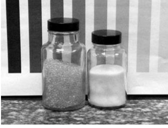
Fig. 2. The jars contain glass spheres and air. In the left jar, the spheres are 4000[\mu\text{m}] wide. In the right jar, which is significantly brighter, the spheres' width is 40[\mu\text{m}] . Thus, tiny spheres create effectively a much higher albedo of a jar, compared to the effect of the large spheres. This is because, in a volume element of a fixed size, there are many more small spheres, leading to many more scattering events. Image taken and adapted from [17], reproduced with permission from SNCSC.
