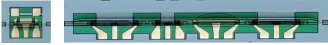
Fig. 2. Microscope picture of the complex coupled DFB (left) with 400 \mu\text{m} total device length and SGDBR (right) with 2650 \mu\text{m} total device length.
