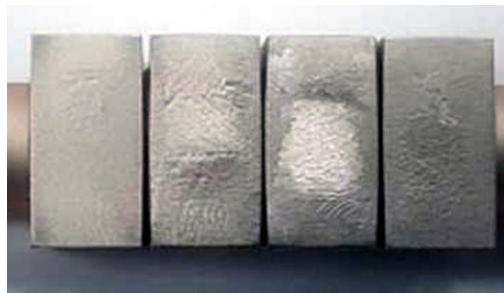
Fig. 8. Demo target ITER-like mock-up ‘‘ENE A 24’’ (8 mm W armor) after 500 cycles at 20 \text{ MW/m}^2 .
