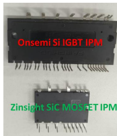
Fig.17. Appearance comparison between SiC MOSFET IPM and IGBT IPM with similar ratings
