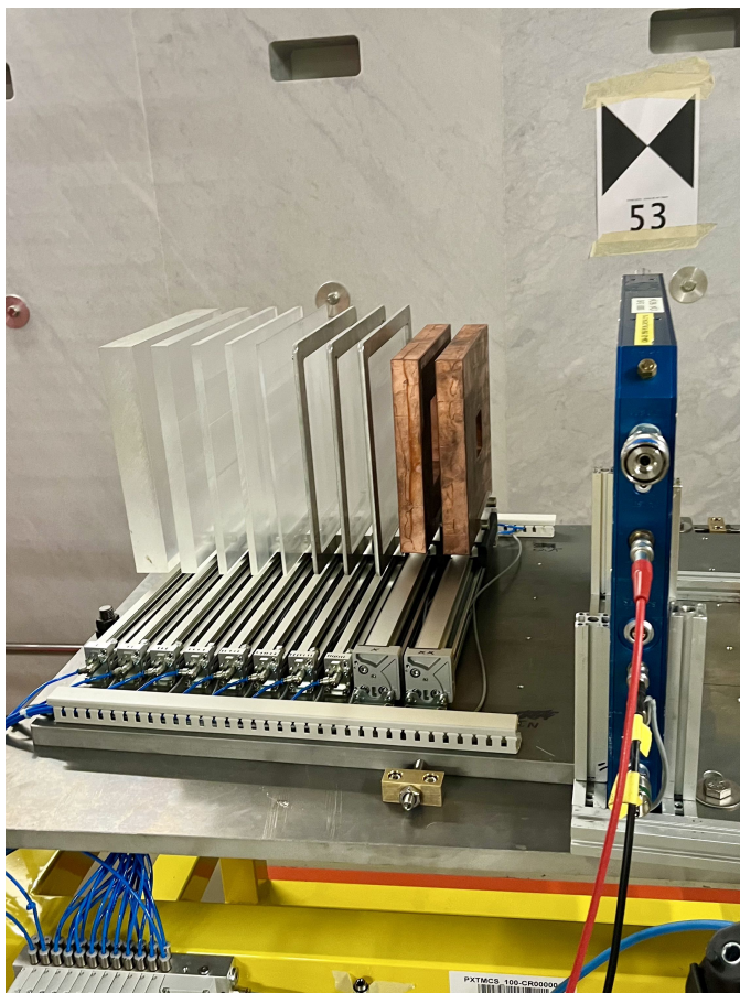
Fig. 2. The PMMA degrader and copper masks system, followed by a parallel-plate ionization chamber, and placed roughly 1 m upstream of the Device Under Test location, which is to the right of the plot.
