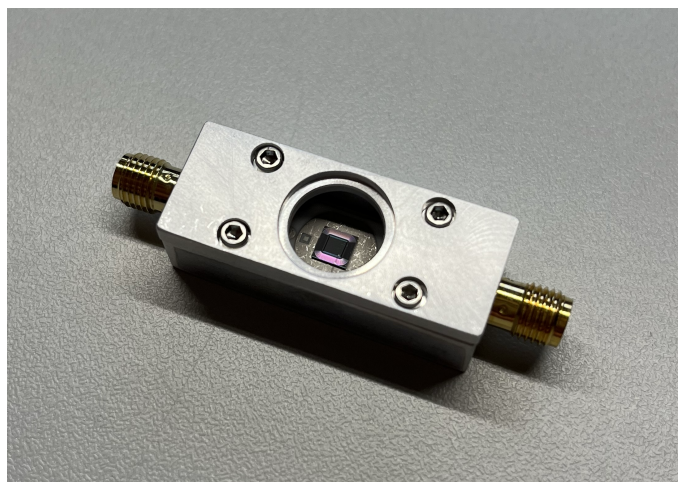
Fig. 2. Silicon diode used for beam characterisation measurements during the HEARTS 2023 ion run.
