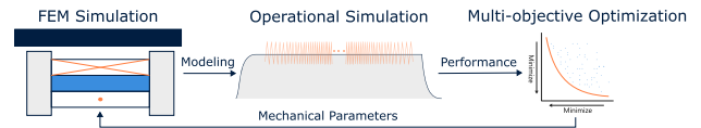
Fig. 1. General sequence of the optimization process involving FEM simulation, model building, levitation simulation, and evaluation using a multiobjective optimization (MOO) algorithm.
