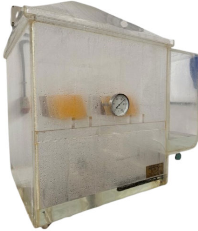
Fig. 1. Experimental setup for the salt spray chamber.
