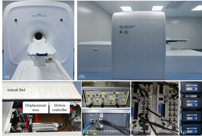
Fig. 3. NHP-MPI system. (a) Front view. (b) Side view. (c) Mechanical displacement device. (d) Preamplifier. (e) and (f) Signal transmission and data acquisition system with a digital-to-analog converter (DAC) and an analog-to-digital converter (ADC). (g) Power amplifiers.
