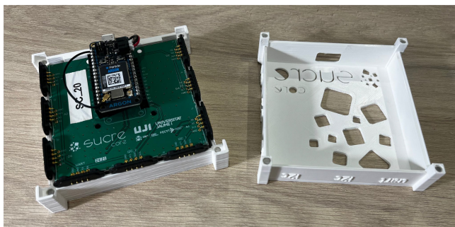
Fig. 4. SucreCore : microcontroller mounted on the custom shield (left) enclosed in the white 3D-printed box.
