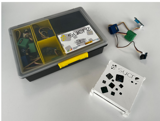
Fig. 3. SucreKit version of Sucre4Stem tool: Sensors (blue), actuators (green), and the SucreCore .
