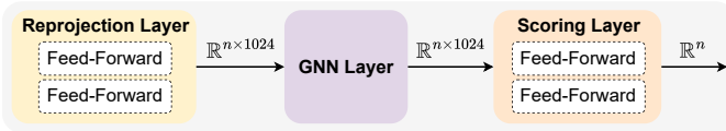
Fig. 3: Overview of our learnable module to model cross-document relationships over the heterogeneous graph. Notably, “GNN Layer” is compatible with various GNN architectures, ensuring our solution’s adaptability and flexibility.
