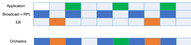
Fig. 2. An Example of Orchestra scheduling 3 repeating slotframes, with EB having the highest priority followed by broadcast (RPL) and unicast (application) cells.
