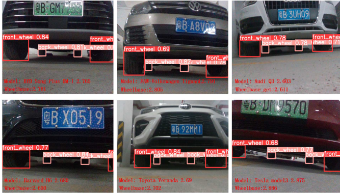
Fig. 7. Performance of the wheel detection and wheelbase calculation
