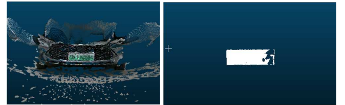
(a) Point cloud of vehicle (b) Point cloud of license plate Fig. 5. The point cloud template of license plate
