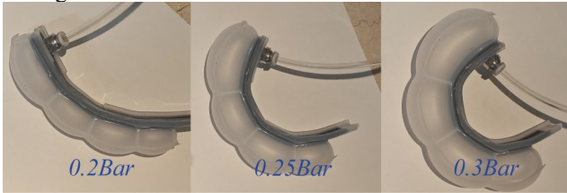
Fig. 10 Shape of the airbag at 0.2Bar, 0.25Bar, 0.3Bar
