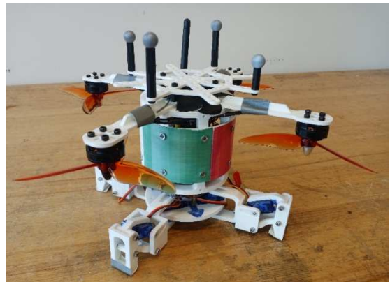
Fig. 1 Multimodal CanBot consisting of Aerial Quadrotor (top) and Terrestrial Quadruped (bottom) mobility modules.
