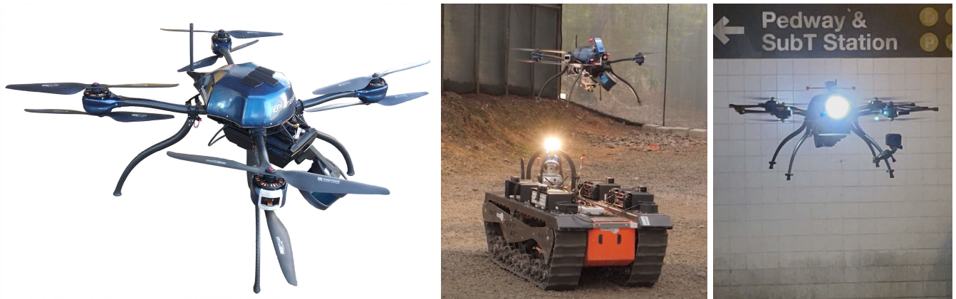
FIGURE 5. Emesent/Aeronavics SubTerra (“Navi”) UAV (left), being launched off the back of an ATR UGV (center), and in flight inside the DARPA SubT finals course (right).
