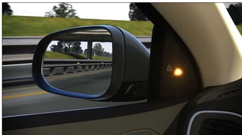
FIGURE 8 Blind spot detection in vehicles. (Source: https://www.extremeaudio.org/ ; used with permission.)
