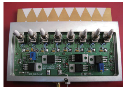
Figure 12 TSPW single RF channel digital beamforming for multibeam antenna array [96].
