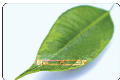
FIGURE 1. Ultrathin oxide TFT on a natural plant leaf substrate.
