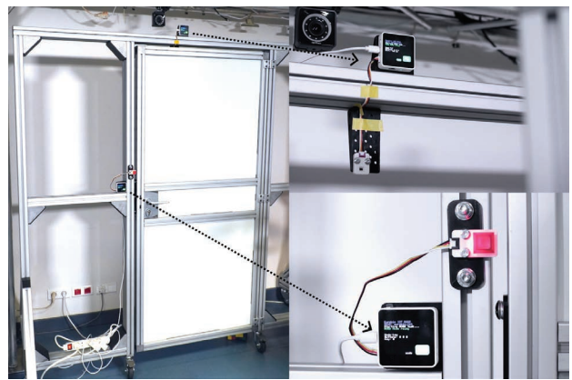
FIGURE 2. Sensorized door, with two sensors (the doorbell and a time-of-flight sensor on top of the frame) that publish the state of the door on ROS2 topics. ROS2: Robot Operating System 2.
