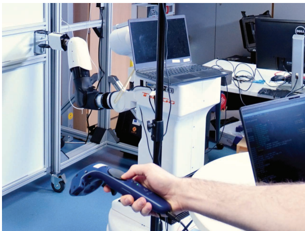
FIGURE 5. INRIA TIAGo-2 teleoperated with the HTC Vive 6-DoF pose controller to open the door.
