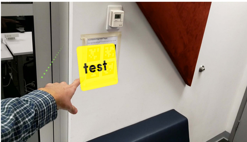
(a) View from HoloLens, in augmented reality, showing a virtual annotation.
