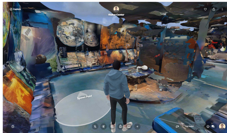
(e) The Visitor Center Museum had many intricate details that were extremely difficult for our smartphone LIDAR scanner to capture, resulting in a very messy looking scan.
