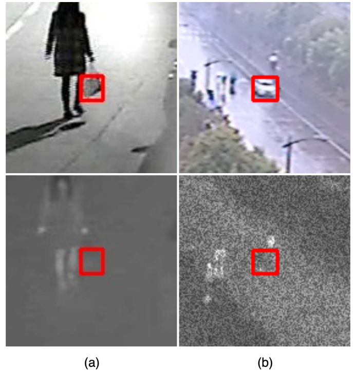
Fig. 2. Illustrative of complementary information for RGB images and TIR images. (a) and (b) are two example frames of the RGB modality and the TIR modality, respectively. As shown in the area marked by the red box, there is remarkable image complementary information between the two modalities, which can improve the accuracy of object tracking.
