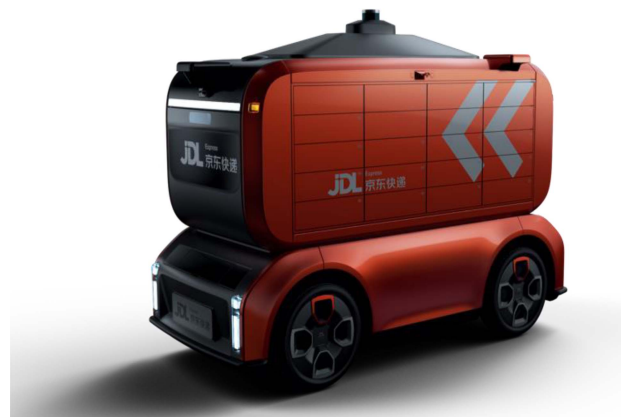
Fig. 5. The 5-th generation of autonomous LMD vehicles developed by JD Logistics.
