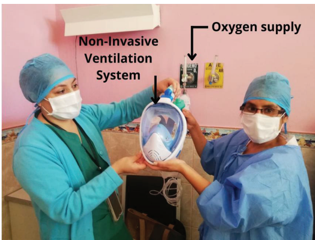
Fig. 11. Test of the snorkel system with oxygen
