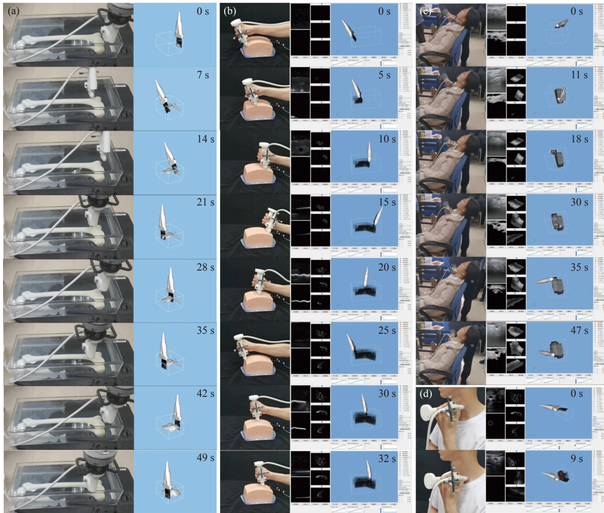
Figure 9 The process of 3D imaging experiments. (a) Femur model; (b) Neck phantom; (c) Human; (d) Human carotid artery.
