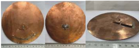
Fig. 5. Photograph of the fabricated dual-mode antenna on air substrate.
