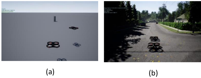
Fig. 2. Unreal environment that was used for training. The left image (a) shows the simple environment used to train the network to identify the target, and the right image (b) illustrates the complex, partially observable environment.
