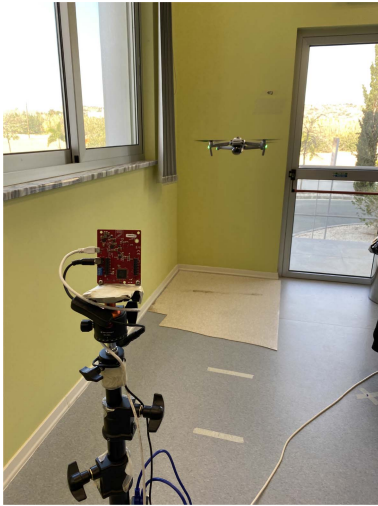
Fig. 4. mmWave 3-DOF precision analysis setup using 3-DOF mmWave sensors.
