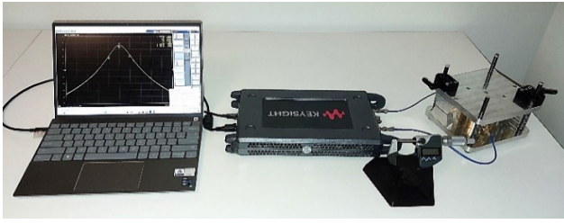
Fig. 3. Measurement setup featuring the 10-GHz Q-SCR prototype (on the right).
