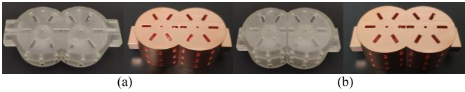
Fig. 7. Manufactured prototypes of the vertically integrated multiband BPFs before and after Cu-plating. (a) Dual-band. (b) Triple-band.
