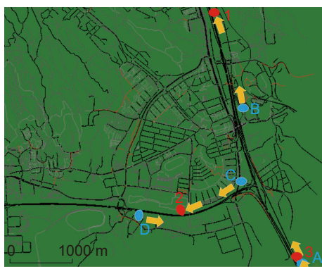
Fig. 1 A part of Gothenburg in SUMO. Blue loops inject traffic, and red loops detect traffic. Traffic detected by the red loop 3 is generated by the blue loop A. Traffic detected by loop 2 is generated by loops A and C. Traffic detected by loop 1 is generated by loops A, B, and D.
