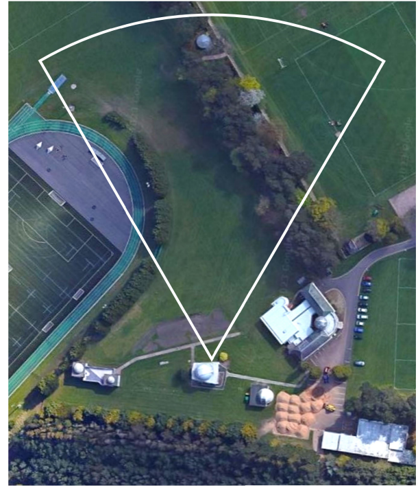
Fig. 19. 60° PPI scan of trihedral and environment at St Andrews Observatory, with aerial image (Google) showing approximate field of regard (note that the trees around the oval running track had been removed prior to the PPI scan).
