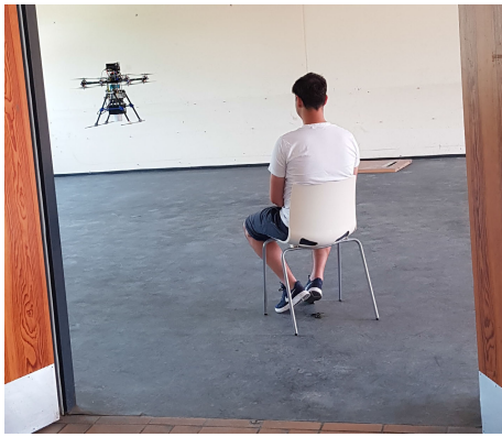
Fig. 10. Photo of measurement with a person and the UAV equipped with rotating radar and LIDAR at TCRH in Mosbach.
