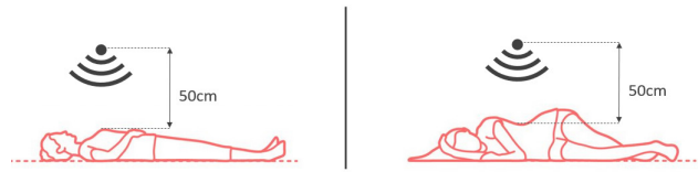
Fig. 4. The left image shows the subject and radar positions in the first part of the experiment (supine position); the right image shows the positions in the second part of the experiment (right lateral decubitus).
