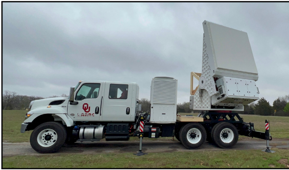
Fig. 1. Photograph of the mobile, fully digital, S-band polarimetric phased array radar called “Horus.” The system consists of 25 panels each with 8 \times 8 dual-polarization elements (1,600 polarimetric elements in total).
