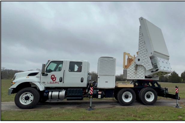
Fig. 1. The fully digital Horus mobile radar, with 25 antenna panels ( 8 \times 8 dual-pol elements each). More details can be found in the Horus System article published in this journal [8].
