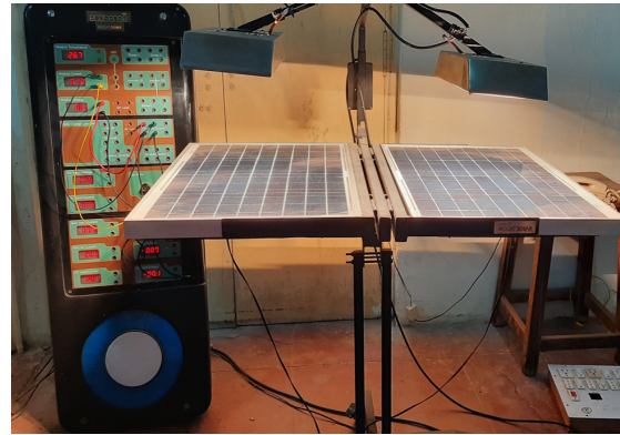
Fig. 6. PV Panel Experimental Setup.
